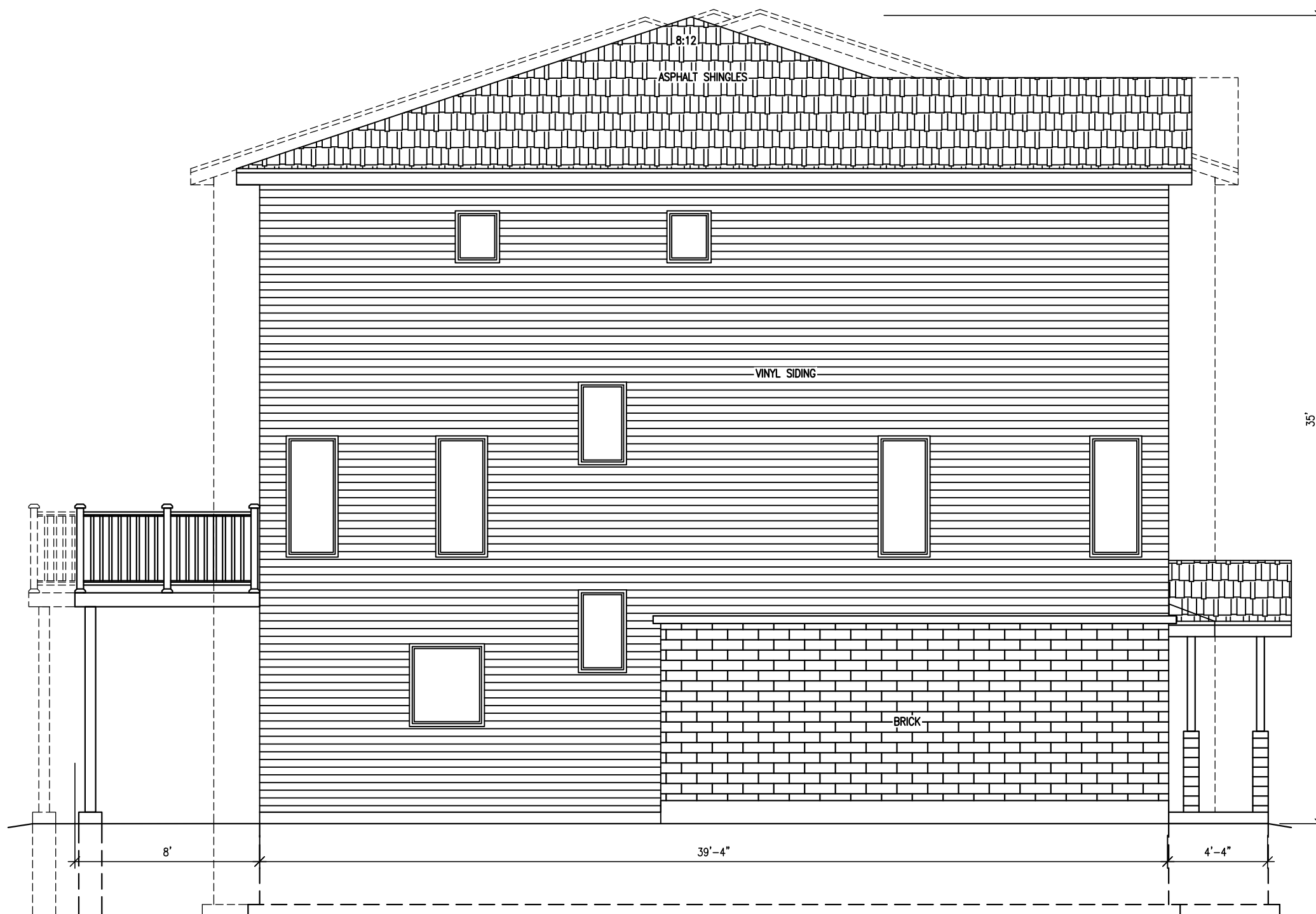
2 LEFT SIDE ELEVATION EL2 SCALE: 3/16"=1'
