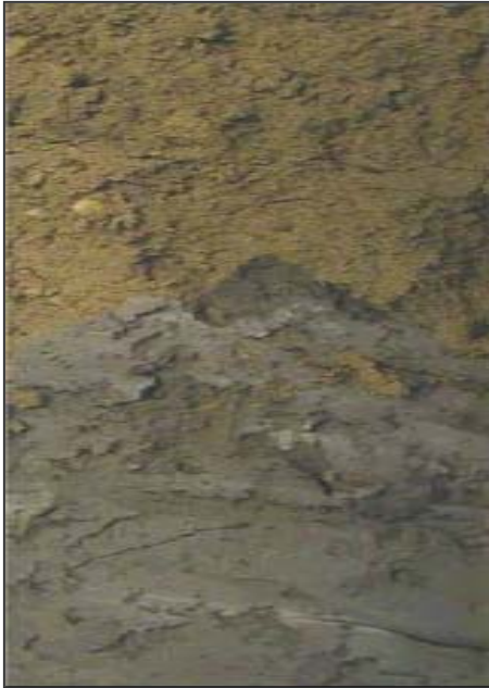
Photograph B1 – Port Stanley Till overlying Maryhill Till in a soil sample from BH2
