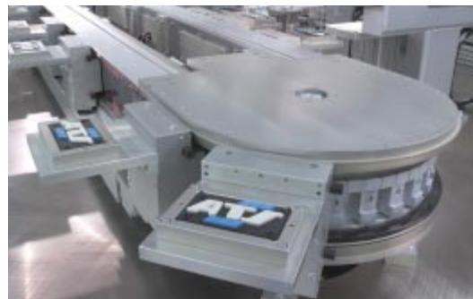
The ATS Supertrak™ is a system that transports components to different workstations – for automated manufacturing processes.
